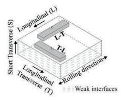
Figure 1 – SE(B) specimens in T-L and L-T orientation following the ASTM classification [13]. Source: Prepared by the authors (2025).
