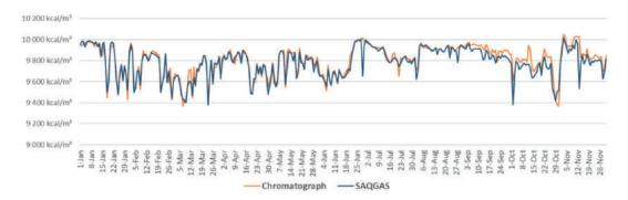
Figure 13 - GCV comparative between computational simulation and chromatograph - Suzano/SP.
