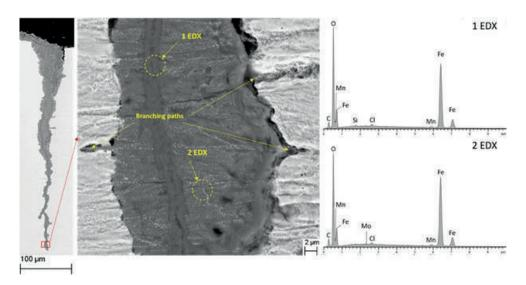
Figure 8 – SEM-BSD cross-sectional images of crack 2 in sample B60 (left, middle). The middle figure is a high-magnification image of the area ensconced within the red rectangle in the left image. The EDX spectra (right) correspond to the dotted yellow circles (spot size of the beam, 2.5 µm) in the middle image.
