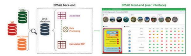
**Figure 2 - PSMS system architecture.** Source: Prepared by the authors (2024)
