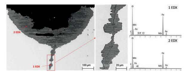
Figure 10 - SEM-BSD cross-sectional images of the crack and pit in sample B3060 (left, middle). The middle figure is a high-magnification image of the area ensconced within the red rectangle in the left image. The EDX spectra (right) correspond to the red arrows (beam spot size: 2.5 µm) in the left image. Source: Prepared by the authors (2025).
