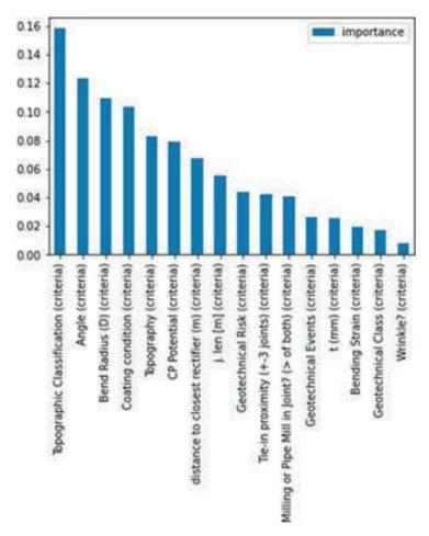
Figure 3 - Ranking of variables based on their importance for C-SCC identification, using the Feature Importance model.
