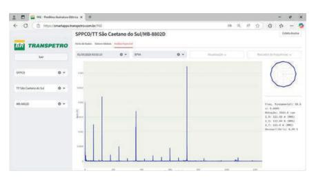
Figure 11 – EPVA and Park Vector graphs in the "Análise Espectral" (Spectral Analysis) tab. Source: Prepared by the authors (2025).
