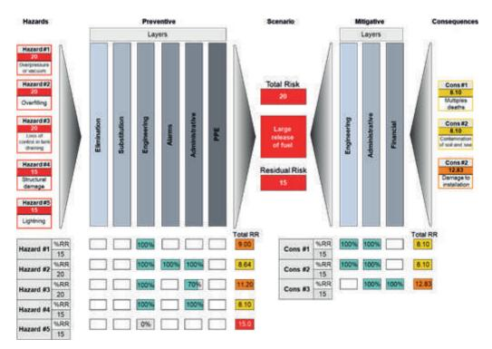
**Figure 4 - Example of dynamic bowtie.** Source: Prepared by the authors (2024)
