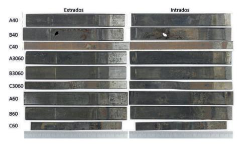
Figure 2 – Photographs of samples after SCC-CO<sub>2</sub> testing. Note the severe corrosion observed in sample B40. Source: Prepared by the authors (2025).
