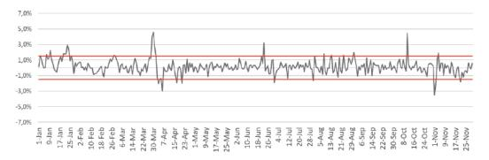
**Figure 10 - Simulation versus Chromatography percentage difference - Volta Redonda/RJ.**Source: Prepared by the authors (2025).
