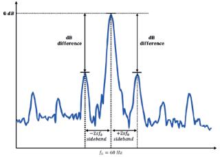
Figure 1 – Illustration of sidebands around the fundamental frequency, characteristic of the broken bar fault mode.
