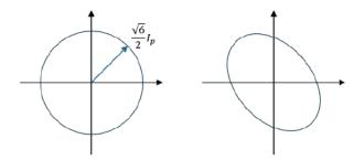
Figure 2 – Park Vector pattern for conditions without and with fault. Source: Prepared by the authors (2025).
