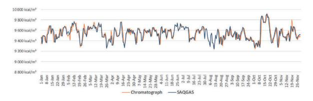
**Figure 7 - GCV comparative between computational simulation and chromatograph – Guapimirim.**Source: Prepared by the authors (2025).
