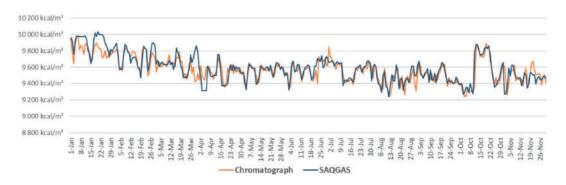
Figure 9 - GCV comparative between computational simulation and chromatograph.
