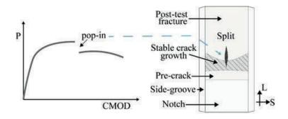
**Figure 2 - Illustration of a pop-in caused by a split.** Source: Prepared by the authors (2025). Inspired in [14].
