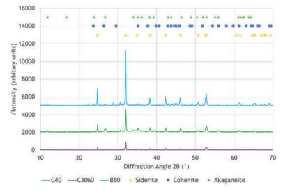
Figure 5 – X-ray diffractograms for surface corrosion scale powders (shown with increasing offset) removed from samples C40 (green), C3060 (magenta), and B60 (blue). Symbols at the top of the plot denote peak locations associated with siderite, cohenite, and akaganeite.
