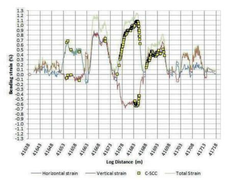
Figure 2 - Results of total, horizontal and vertical bending strain for an investigated site. The squares represent the SCC colonies verified at this site.
