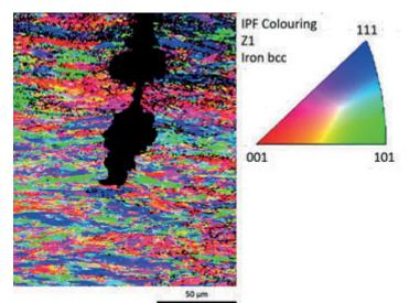
Figure 11 - EBSD orientation image map with inverse pole figure (IPF colouring) of the crack tip in sample B3060. Significant concentrations of elongated grains are visible adjacent to the crack. Several grains oriented along the [001] direction are located around the narrow channel of the crack between wider crack sections.
