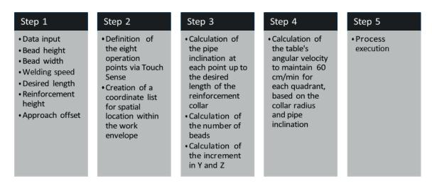
Figure 3 - Flowchart of the trajectory planning used for the reinforcement collar deposition.
