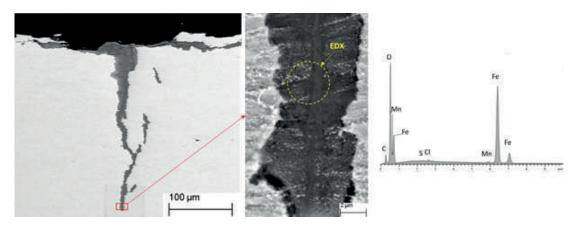
Figure 6 – SEM-BSD cross-sectional images of crack 1 in sample B60 (left, middle). The middle figure is a high-magnification image of the area ensconced within the red rectangle in the left image. The EDX spectrum (right) corresponds to the spot size of the beam (2.5 μm, dotted yellow circle) in middle image. Source: Prepared by the authors (2025).
