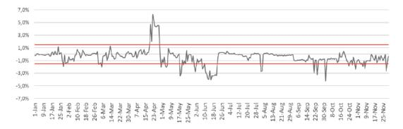
Figure 12 - Simulation versus Chromatography percentage difference - Caçapava/SP.
