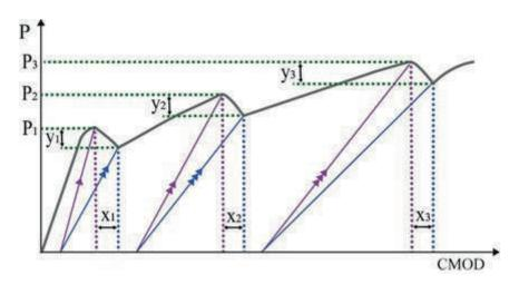
**Figure 6 - Determination of parameter** *F***.** Source: Prepared by the authors (2025). Inspired in <sup>[2]</sup>.
