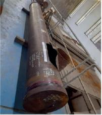
Figure 3 - Fracture surfaces and rupture locations in specimens after internal pressure burst test. Prepared by the author (2025)
