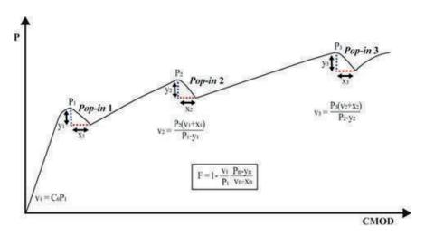
Figure 3 - Exaggerated pop-ins and illustration of the evaluation of F.
