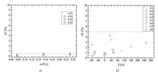
Figure 3 - Results of a) specimen compliance change obtained by numerical simulation and b) compliance changes obtained by experimental test.
