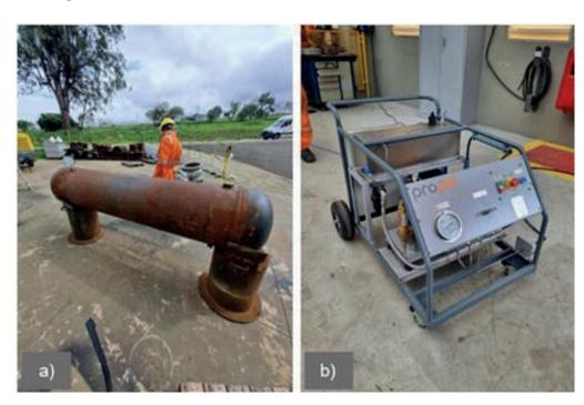
Figure 4 – a) Balloon for testing; b) Hydrostatic pump.
