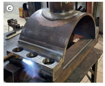
The measurements performed on the clamp focused on the diameter of the flat section, width, and thickness of the reinforcements. The results of these measurements are detailed in Table 1. It was found that all measurements were within the initially defined tolerances, with a low standard deviation.
