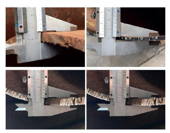
Figure 2 - Wall Thickness Profiles at Clock Positions 12h, 6h, 9h, and 3h.
