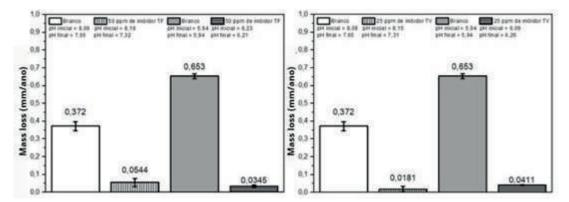
Figure 3 - Mass loss of the average of triplicates after 24 hours of immersion of 1020 carbon steel in different media (a) with and without TF inhibitor and (b) with and without TV inhibitor.
