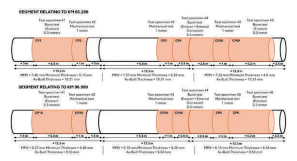
**Table 1 – Segmentation of Pipe Specimens Extracted from Hydro's 24-inch Slurry Pipeline.**Prepared by the author (2025)
