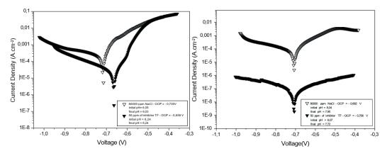
Figure 4 - Potentiodynamic polarization with and without addition of TF inhibitor (a) pH 6 and (b) pH.
