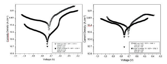
Figure 5 - Potentiodynamic polarization with and without addition of TV inhibitor (a) pH 6 and (b) pH 8.
