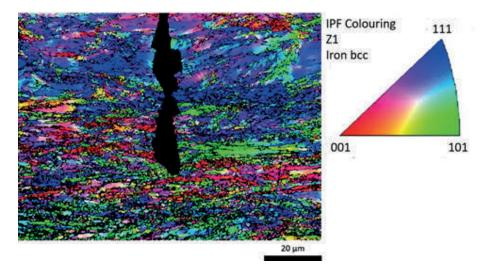
Figure 9 - EBSD orientation image map with inverse pole figure (IPF colouring) of the tip of crack 2 in sample B60. Fine grains are visible adjacent to the crack. A region of grains oriented along the [111] direction is visible approximately 35-40 μm above the crack tip. Source: Prepared by the authors (2025).
