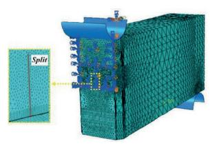
Figure 4 – Meshing and boundary conditions of FEM models.
