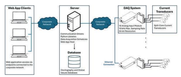
**Figure 7 – Schematic of the online electrical signature collection system.**Source: prepared by the authors (2025).
