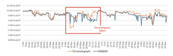
Figure 11 - GCV comparative between computational simulation and chromatograph - Caçapava/SP.
