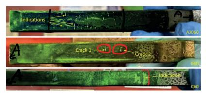
Figure 4 – Magnetic particle inspection (MPI) results for samples A3060, B60, and C60. Indications are visible on the surface of the samples as denoted by the yellow arrows. Cracks were identified in B60. The letter A denotes the datum. No indications were detected on other samples. Source: Prepared by the authors (2025).
