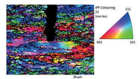
Figure 7 - EBSD orientation image map with inverse pole figure (IPF colouring) of the tip of crack 1 in sample B60. Fine grains are visible adjacent to the crack and relatively large grains are present in front of the crack. Source: Prepared by the authors (2025).
