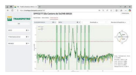
Figure 10 - MCSA graph in "Análise Espectral" (Spectral Analysis) tab.
