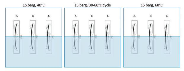
Figure 1 – Three samples were loaded in 4-point bend configurations and half-submerged in 3.5 wt.% NaCl solution in each deaerated CO2-containing autoclave. Tests were carried out at 40°C for 180 days, 30-60°C for 100 days, and 60°C for 128 days. The pressure was 15 barg in all tests.
