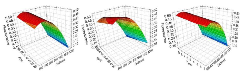
Left: Fluorescence as function of sediment and flow with light 50 %. Middle: Fluorescence as function of light and sediment with flow 0.7 m/s. Right: Fluorescence as function of time and sediment with flow and light constant at 0.7 m/s and 50 %, respectively (Source: Peregrino Marine Calcareous Algae - PEMCA, supported by Statoil and ANP)
